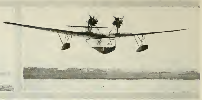
Rohrbach Rostra with two Jupiter air-cooled engines
